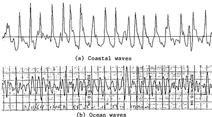
Figure 1: Comparison of coastal and ocean wave profile
