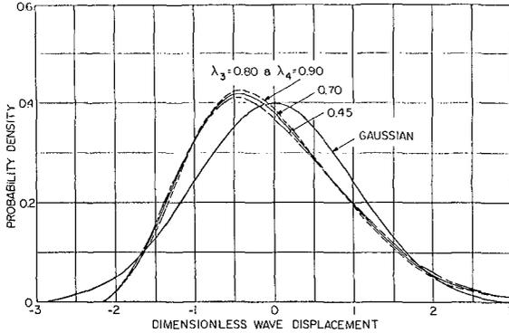
Figure 10: Comparison between normal probability distribution and non-Gaussian distribution with  $\lambda_3 = 0.80$  and  $\lambda_4 = 0.45, 0.70,$  and  $0.90$
