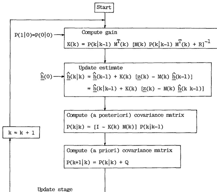
Fig. 6.— Algorithm of Kalman Filtering
