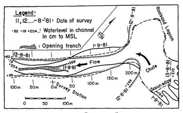
FIGURE 4: Breaching at "Rooisand", II August 1981
