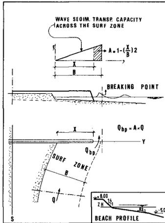
FIG 14 - Bypassing process of
