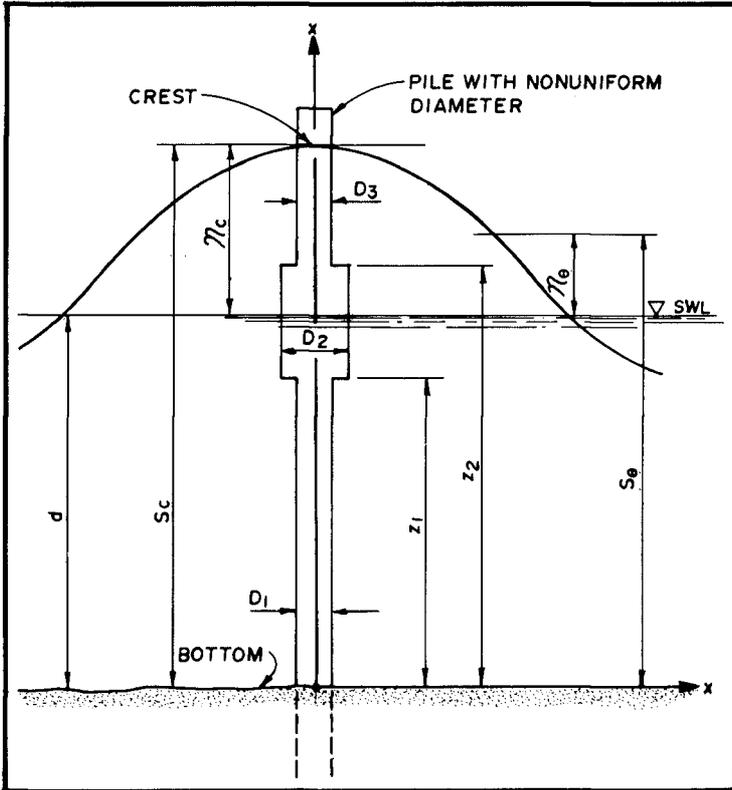
Figure 1. Definition Sketch for a Pile with Three Diameters.
