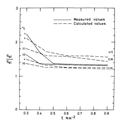
FIGURE 5. Comparison between the calculated and measured ratios of bed load transport rates,  $\mathbf{q}_{\mathbf{s_l}}$ , and  $\mathbf{q}_{\mathbf{s_l}}$ , induced respectively by turbulent and laminar flows, as a function of mean bed shear stress.
