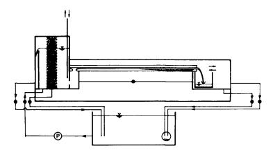
FIGURE 1. Laminar flow channel used to measure bed load sediment transport induced by a laminar boundary layer formed between closely spaced parallel plates.
