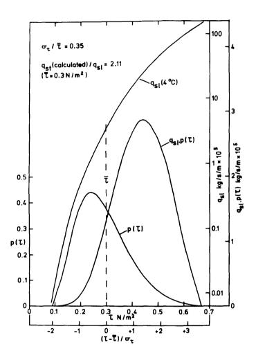
FIGURE 4. Sample illustration of the method of calculating bed load transport rate produced by a turbulent flow,  $q_{st}$ , at a particular mean bed shear stress  $\bar{\tau}$  of  $0.3\text{N/m}^2$ , from the laminar flow transport relationship,  $q_{st}$ , and the probability distribution,  $p(\tau)$ , of the fluctuating bed shear stress,  $\tau$ , induced by the turbulent flow.
