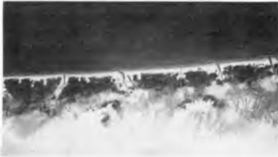
Figure 11. Vertical aerial photograph showing irregular periodicity of washover channel spacing on Central Padre Island (photo taken 8/20/80).
