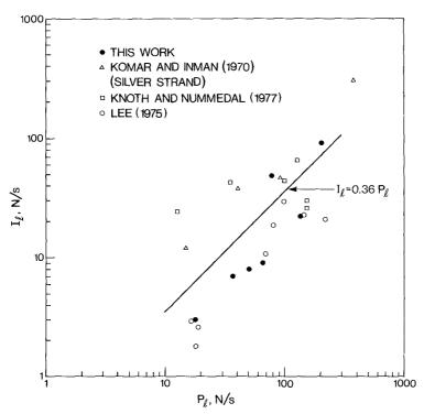
FIGURE 2. IMMERSED WEIGHT SUSPENDED SEDIMENT DISCHARGE vs LATERAL THRUST × PHASE SPEED.
