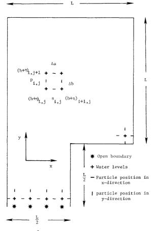
Figure 3. Configuration of Semi-enclosed Basin
