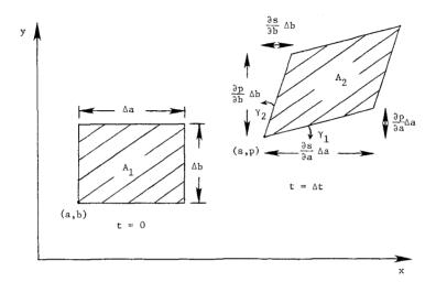
Figure 1. Deformation of a Fluid Element
