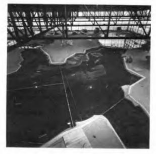
Figure 4: Hydraulic model of the Oosterschelde The boundary conditions of the models were obtained from extensive measurements in the prototype (fig. 5).
