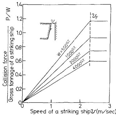
Fig. 12 Estimated impact forces at the bow collision
