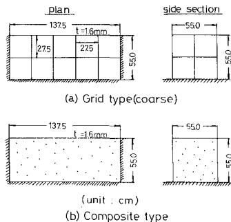
Fig. 14 Model dimensions of the coarse grid-type and the composite-type
