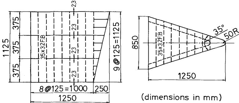
Fig. 7 One-fourth scale bow model of 500 G.T. ship
