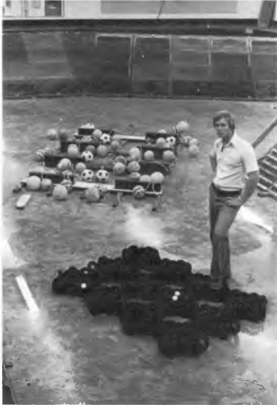
Plate 3. One-quarter scale model of TF-Breakwater in drained wave tank at Canada Centre for Inland Waters (model of Goodyear Breakwater in foreground).
