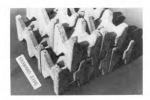
Fig. 5.- N-Shaped Blocks in Two Layers
