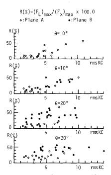
Figure 7. Ratio of the maximum lift force to the maximum in-line force versus rmsKC number(in cases of plus inclinations).
