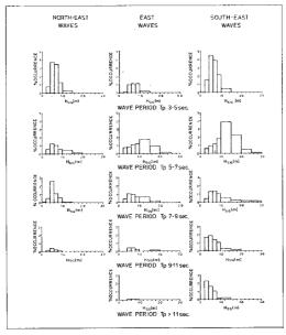
Fig. 7 Wave Height/Period/Direction Occurrence
