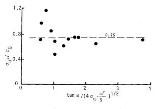
Fig. 1 Ratio of turbulent to wave-induced velocity intensity (Thornton, 1978)
