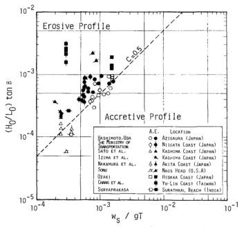
Fig. 13 Applicability of the model to the prototype.
