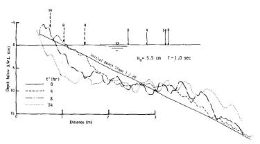
Fig. 7 Profile changes of erosive beach (sand).
