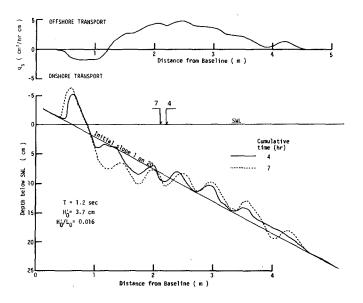
Fg. 9 Method for determining transport rate.
