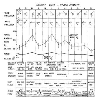
Figure 4: The annual Sydney wave climate and beach form. The wave height and energy is based on a nine years (1971-79) monthly mean of daily wave conditions (M.S.B. data). The stradling line and bars equal <sup>±</sup> one standard deviation. The beach response through the year is reflected in the beach stability, surfzone type and beach form. The plan view of beach form illustrates the beach response typical open beach responding fully to the above conditions (from Short and Wright, in press).
