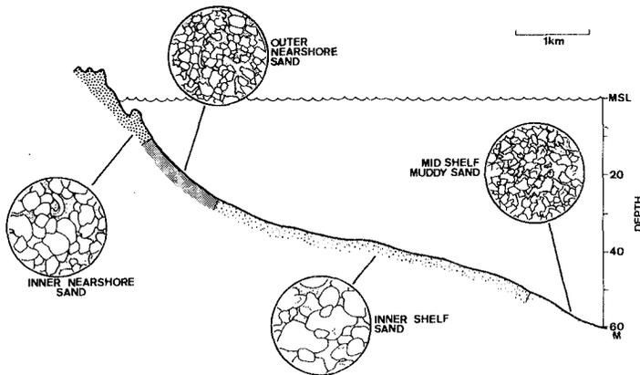
Figure 2. Typical, concave-up sea bed profile showing normal arrangement of sediment types. Lithologies (insets) illustrating grainsizes and shapes are drawn from photomicrographs at the same scale; stippled areas are open spaces.
