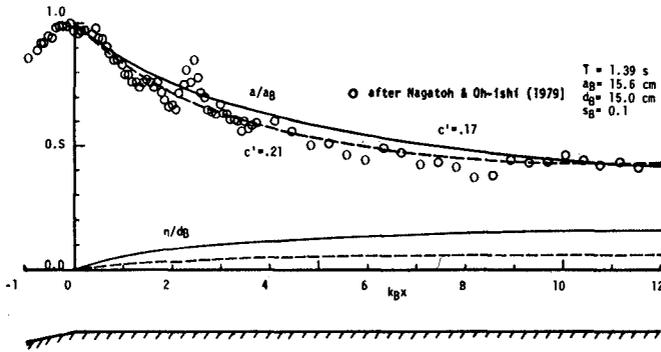
Figure 4 Comparison with experiment ( constant depth beach )
