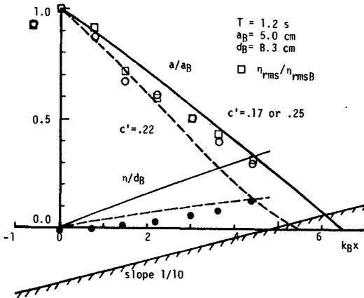
Figure 5 Comparison with experiment ( uniformly sloping beach )
