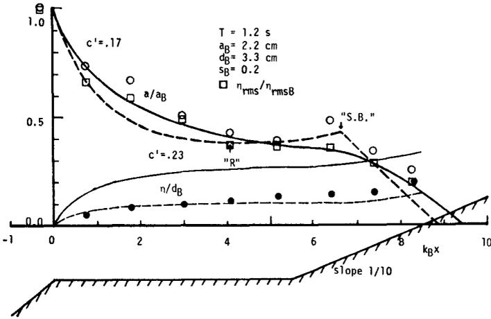
Figure 6 Comparison with experiment ( step type beach )
