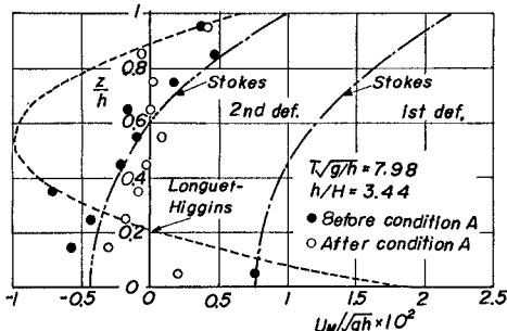
Fig. 10 Comparison of mass transport velocity in normal wave tank with theoretical curves
