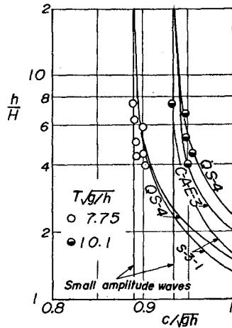
Fig. 7 Comparison of wave celerity with theoretical curves
