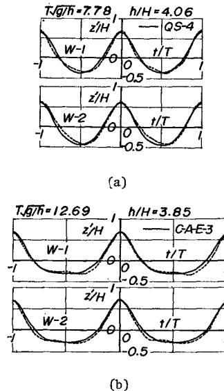
Fig. 6 Comparison of wave profile with theoretical curves
