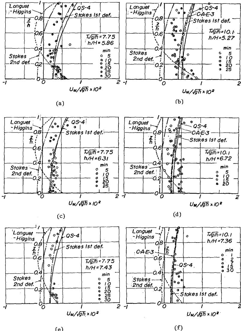
Fig. 8 Comparisons of mass transport velocity with theoretical curves (1)
