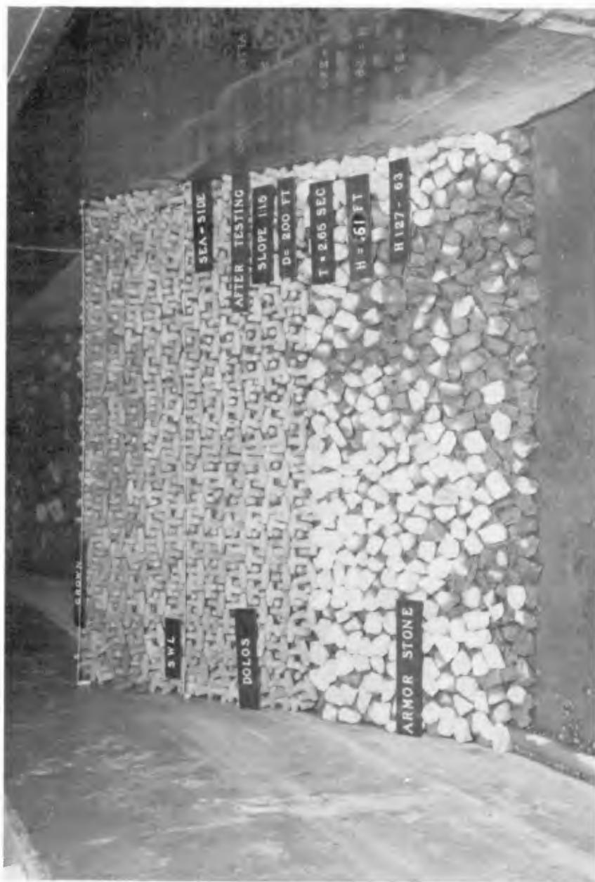
Photograph 9. Pattern 3 after attack of 2.65-sec, 18.5-cm waves
