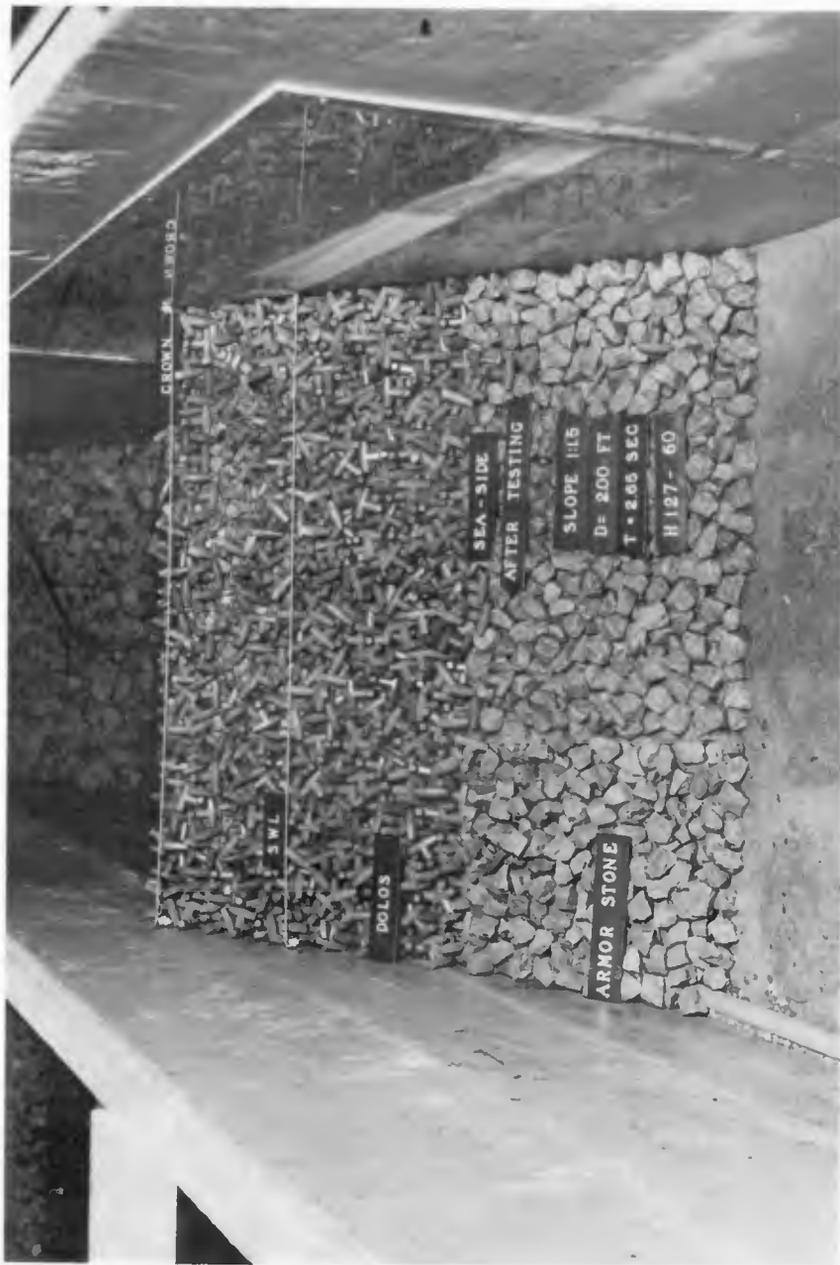
Photograph 3. Pattern 1 after attack of 2.65-sec, 18.5-cm waves
