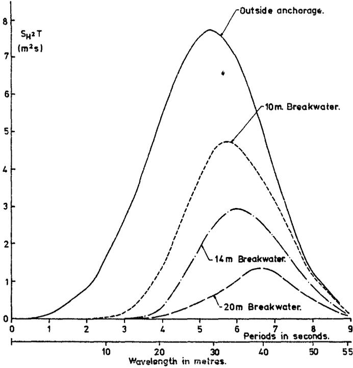
fig 10: Performances for three possible breakwaters at Gigha
