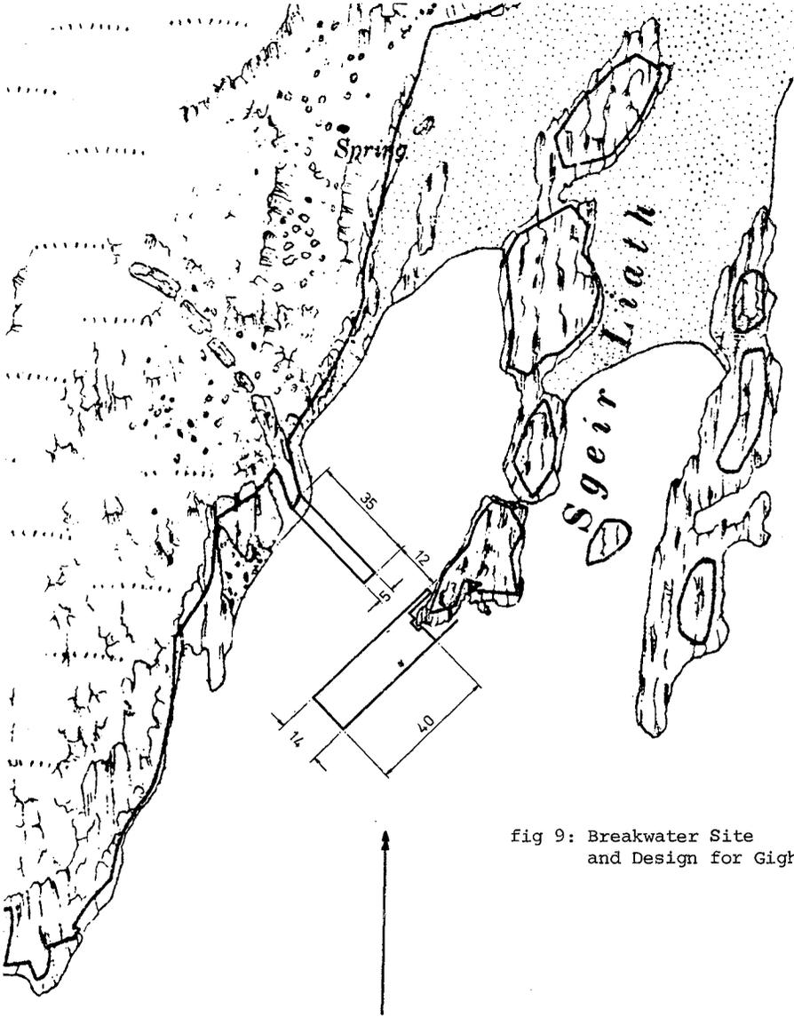
fig 9: Breakwater Site and Design for Gigha
