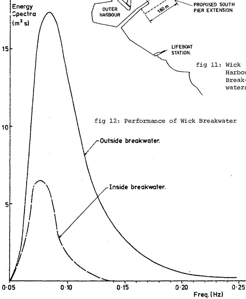
fig 12: Performance of Wick Breakwater
