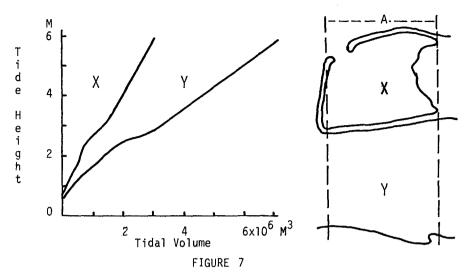
The diagram on figure 7shows the volume of water flowing in the harbor as well as the total volume of water that would otherwise flow through the cross-sectional area A. Less than half the initial volume of water is now flowing over the harbor area. It disrupts the hydraulic equilibrium that used to prevail. Although water is flowing faster at the very entrance of the harbor, the water mass is more tranquil and sedimentation is favored.
