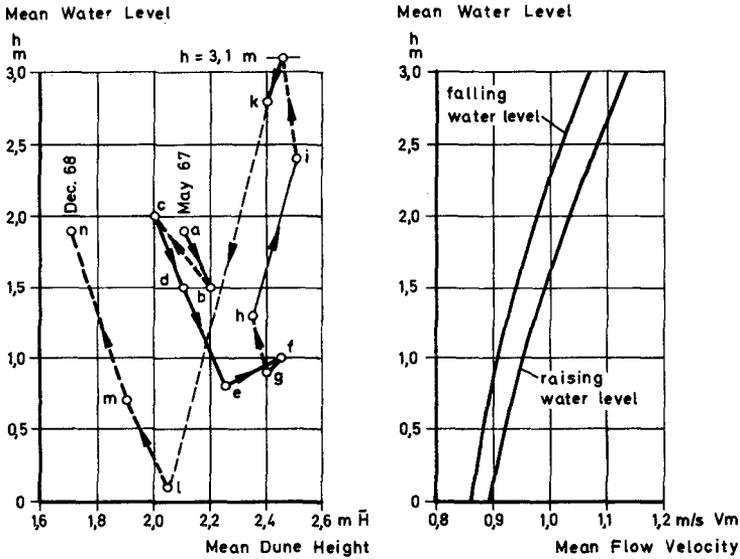
Fig. 8 Mean Dune Height, Flow Velocity and Water Levels in the Rio Paraná (STÜCKRATH, 1969)
