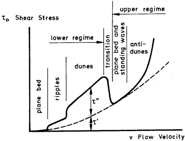
Fig. 1 Bed Shear Stress, Flow Velocity and Bed Forms
