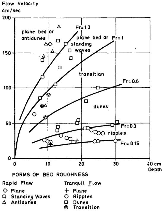
Fig. 6 Flow Velocity, Water Depth and Bed Form (SIMONS and RICHARDSON, 1960)
