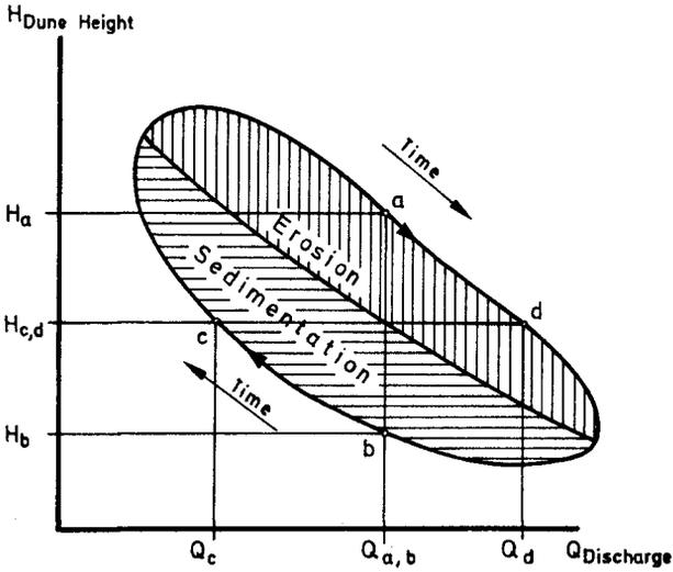
Fig. 4 Schematic Dune-Height Discharge Curve for River Weser
