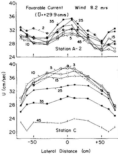
Fig. 3 Lateral current distribution in a case of favorable current.
