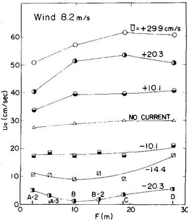
Fig.5 Values of surface current velocity  $u_0$ .
