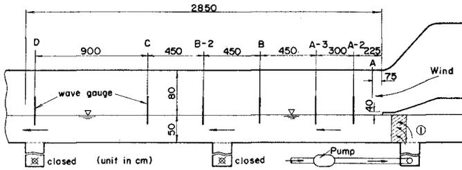
Fig. 2. A side view of the test section
