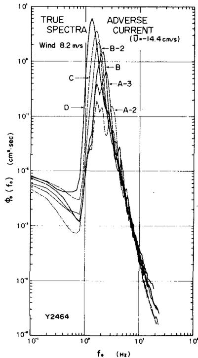
Fig. 8 True spectra ;  $\bar{U}=-14.4$  cm/sec, Wind = 8.2 m/sec.
