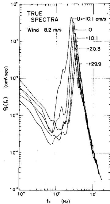
Fig. 10 True spectra under different current conditions.
