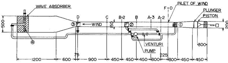
Fig. 1. A plan of the wind-wave channel
