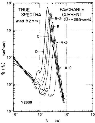
Fig. 7 True spectra ;  $\bar{U}=+29.9$  cm/sec, Wind = 8.2 m/sec.
