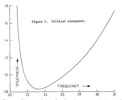
If we consider a particular situation of a narrow tank of length 4m, with a beach of slope  $\alpha = 0.1$ , the numerical integration of the above expression leads to the graph (fig. 1) of the wave steepness at the wavemaker. The damping for the standing wave was taken to be constant  $v = 0.01s^{-1}$ , and the damping for the progressive waves was calculated using the formula
