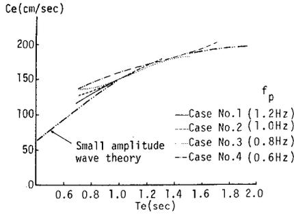
Fig.9 Best fit curves of wave velocity  $\sim$  wave period relations for measured data
