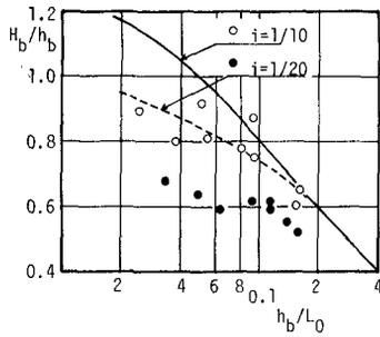
Fig.19 Relations between  $H_b/h_b$  and  $h_b/L_0$  for regular waves
