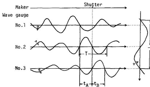
Fig.2 Definition of wave period and wave velocity
