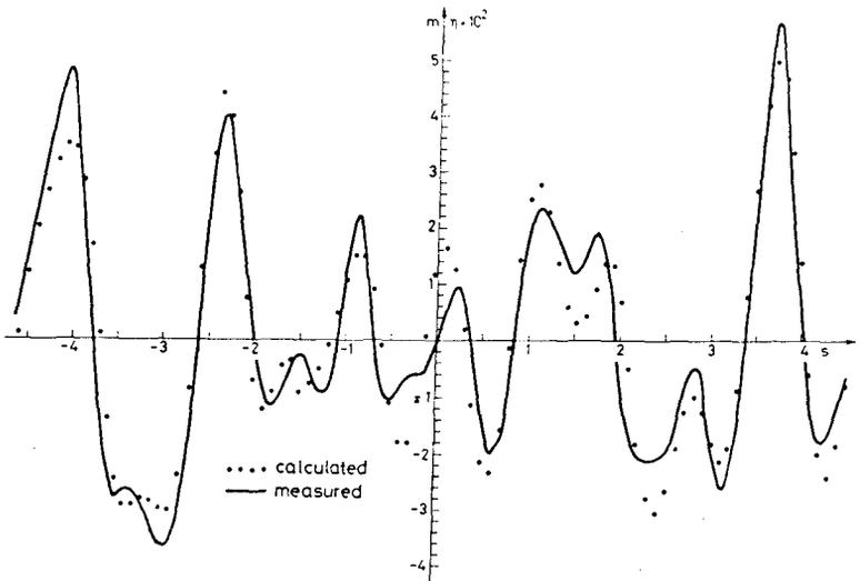
Fig. 5 Calculated and measured elevations at  $x = 8.98$  m
