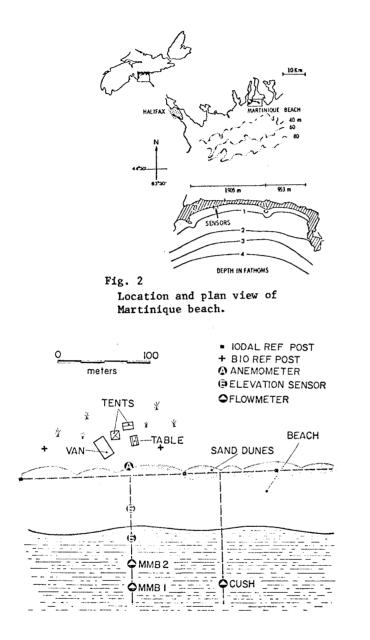
Fig. 3 Placement of sensors.
