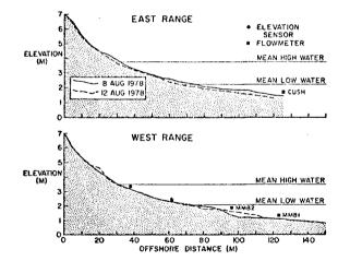
Fig. 7 Beach profiles before and after storm for both ranges. MMB2 was buried by the storm.
