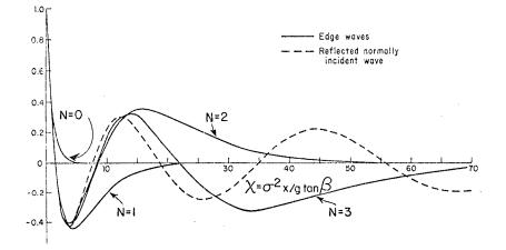
Fig. 1 Offshore dependence f (x) for edge wave modes 0, 1, 2, and 3, and or normally incident reflected wave.
