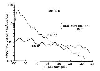
Fig. 10 Example onshore velocity spectra from calm conditions (run 12) and from storm conditions (run 25).
