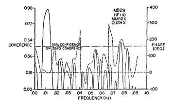
Fig. 12b Coherence and phase between the onshore velocities of the MMB2 and Cush for run 29. The 100 second peaks in figure 12a are seen to be highly coherent with a phase of 0<sup>°</sup>.
