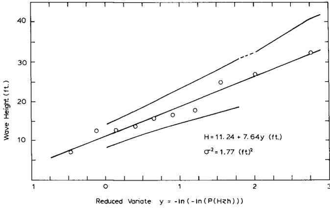
FIG. 6 LINE OF BEST FIT USING GUMBEL'S DISTRIBUTION FOR SIGNIFICANT WAVE HEIGHTS FROM 10 STORMS AFFECTING THE HAWAIIAN ISLANDS FROM 1947 THROUGH 1961 HINDCASTS BY MARINE ADVISORS (1964)
