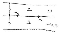
Figure 2: Schematization of Interfacial Transport
