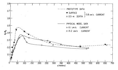
Fig. 13. Comparison of Centerline Temperature Decay from Physical-model and Prototype Data for D. C. Cook Unit 1
