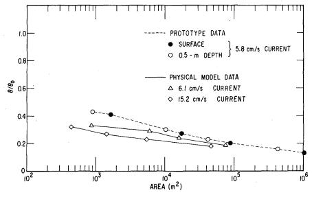
Fig. 14. Comparison of Isotherm Areas from Physical-model and Prototype Data for D. C. Cook Unit 1
