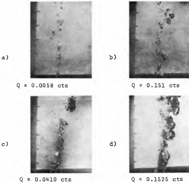
Fig. (7). Effect of Air Flow Rate on Bubble Size in the Transition Zone
