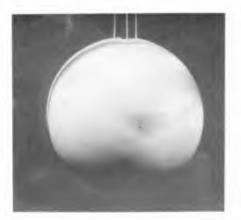
Figure 3. Dye streak produced by two cycles of motion showing circulation proceeding over the top of the sphere at  $\pi d_0/D = 3.2$ . Waves progressing from left to right.
