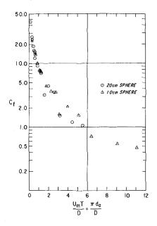
Figure 7. Measured drag coefficients,  $c_f$ , against the inverse of the Strouhal number,  $u_m T/D = \pi d_0/D$ , where  $u_m$  is the maximum horizontal particle velocity in the undisturbed wave; T is the wave period and  $d_0$  is the orbital diameter.
