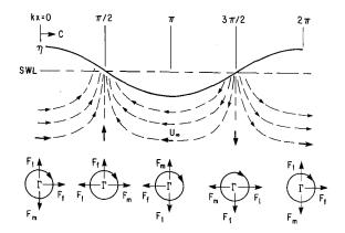
Figure 11. Phase relationships between drag,  $F_f$ , the inertia force,  $F_m$ , and lift,  $F_\ell$ , relative to the wave profile when a circulation,  $\Gamma$ , in the sense of the orbital motion is present.
