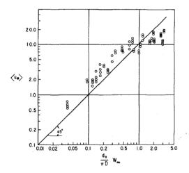
Figure 10. Streaming velocities  $\langle u_{\theta} \rangle$ , measured around the vertical equator of the sphere against ( $d_0 \ w_{\omega}/\pi D$ ) where  $w_{\omega}$  is the amplitude of the vertical particle velocity in the undisturbed wave. Velocities are expressed in units of cm/sec.
