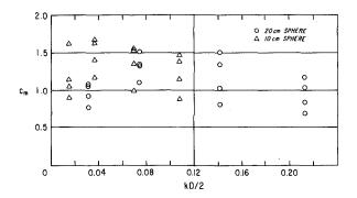
Figure 12. Apparent inviscid inertia coefficients,  $c_m,$  obtained by correcting measured values of  $c_m\,$  for the horizontal component of lift.
