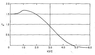
Figure 1. Spherical deep water scattering solution for the inertia coefficient,  $c_m$ , after Havelock (1954), where k is the wave number =  $2\pi$ /wave length; D is the sphere diameter.
