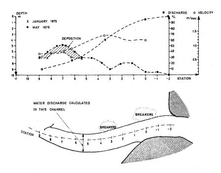
Figure 3. Sedimentation and Ebb Discharges in the Lee of the Breakwater
