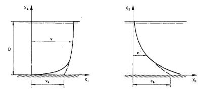
In the following introduction to the basic equations,  $\mathbf{x}_1$  is the horizontal coordinate and  $\mathbf{x}_2$  is the vertical coordinate. The vertical distribution of concentration is considered in two situations.
