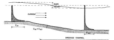
As the flow passes the side of the channel, its velocity changes and therefore the total sediment load, carried as bed load and suspended load, changes accordingly.
