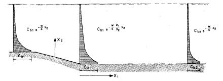
At the toe of the side slope of the channel the approximation is made that the bottom concentration is unchanged, but the concentration profile is stretched with the same ratio as the depth is changed, i.e.  $D_1$ . Therefore the concentration is given by
