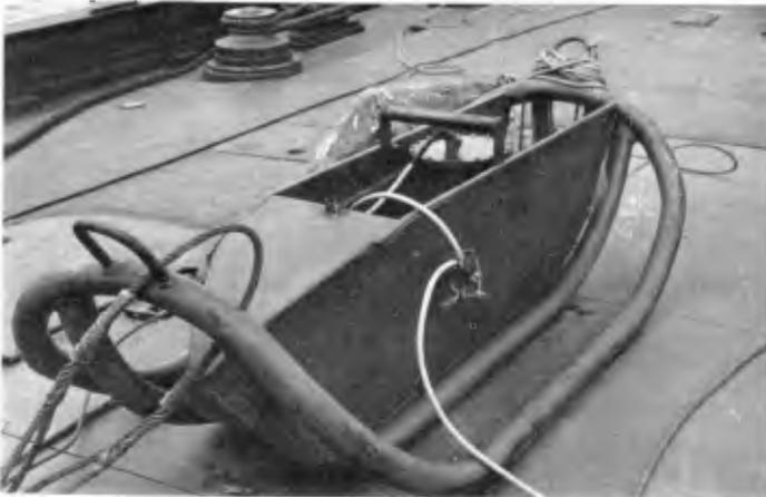
Fig. 4: The new measurement sledge, lateral view
