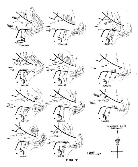
In the period 1956-1959 the northern jetty was built to a point of 2,150 feet seaward of the reference line referred to earlier. At this stage the bar depth was unchanged but the bar was in the form of an isolated shoal with deeper water between the shore and its two ends. The bed of the small bay between the entrance and Wooli Head had deepened by about 10 feet - see fig. 6.
