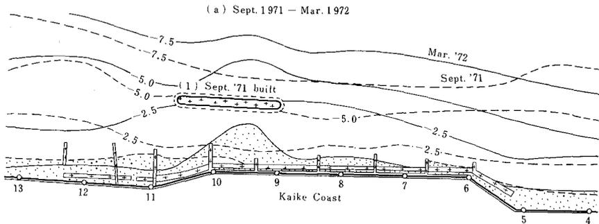
Fig.15 Changes of shoreline and equi-depth line before and after the construction of the No.1 detached breakwater at Kaike.
