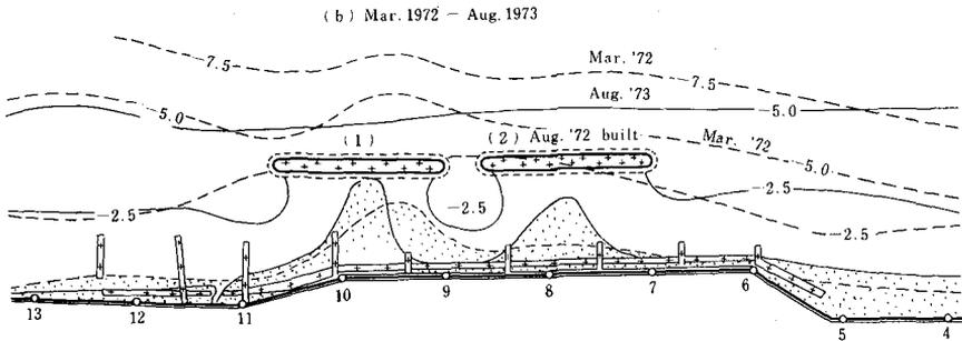
Fig.16 Changes of sea bed after the construction of the No.2 breakwater.
