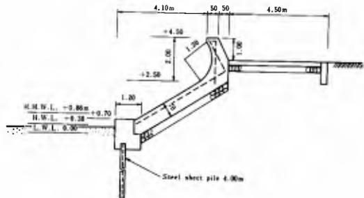
The profile of seawall restored by the local government was an inclined-face type seawall with sandtight cutoff wall by steel sheet pile as shown in Figure 11.
