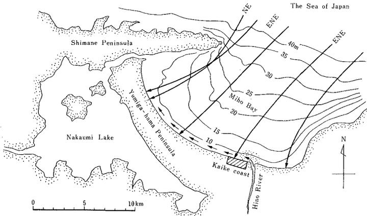
Fig.2 The longshore current formed the Yumiga-hama Peninsula in ancient times, and now-a-days it erodes the Kaike coast on account of reduction of sand supply from the Hino River.
