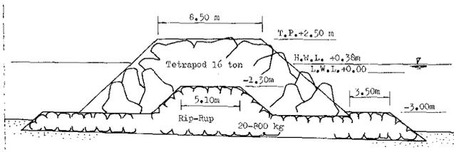
Fig.14 Cross-section of the detached breakwater at Kaike.
