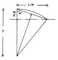
Fig. 2. Approximation of Centrifugal Effect
