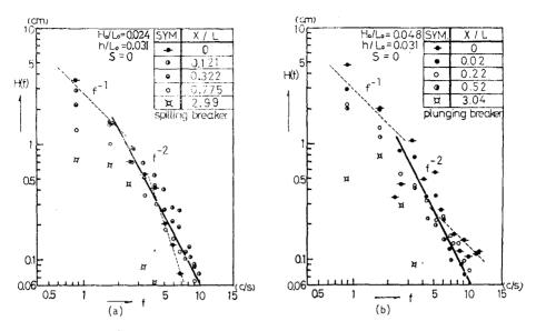
Fig. - 5. Variation of wave height spectrum. (S=0) ( Predominant components )
