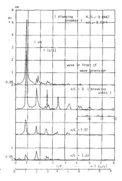
Fig.-2. Variation of wave height spectrum. (S = 0)
