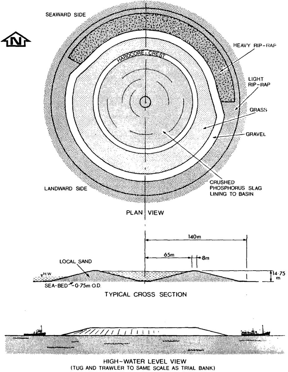
Figure 2. Details of Offshore Trial Bank
