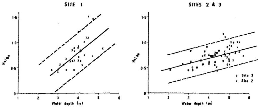
Figure 4. Variation of wave height with water depth
