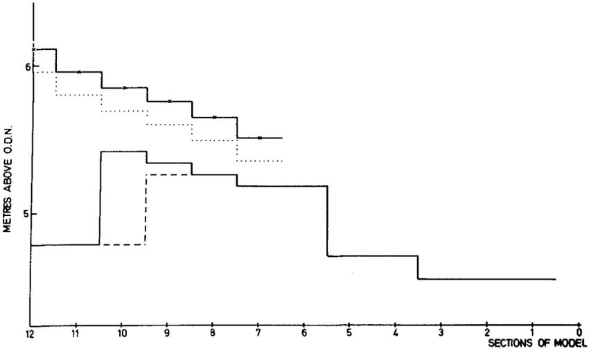
Figure 2. The lowest bank level at each section of the model. The levels in sections 1-6 are approximately those of 1953, by 1970 the bank levels here were sufficiently high that no flooding occurred in the surges used in the study.
