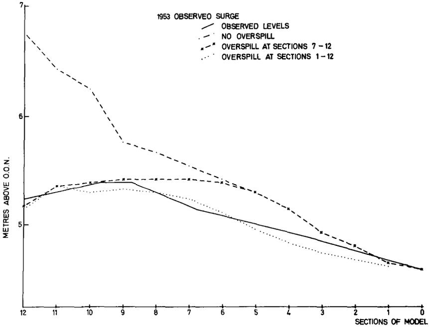
Figure 3. Maximum water levels reached along the river, bank levels I (1953) for overflow at all sections, I (1970) restricting the flooding to the upper river.
