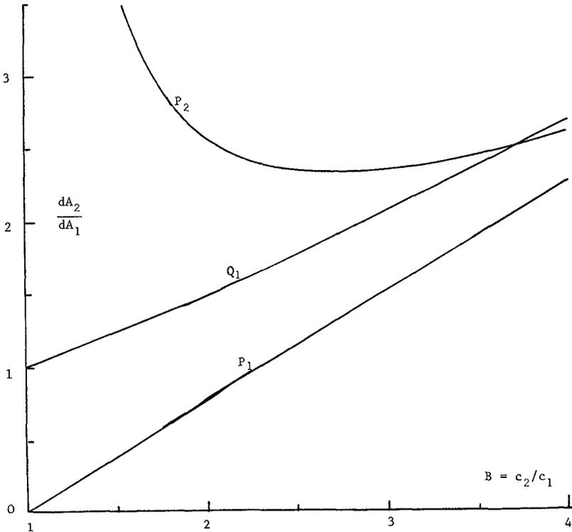
Figure 4. The relative change in volume when a small amplitude wave meets a bore. The curves are labelled with the corresponding Riemann invariants of the incident wave.
