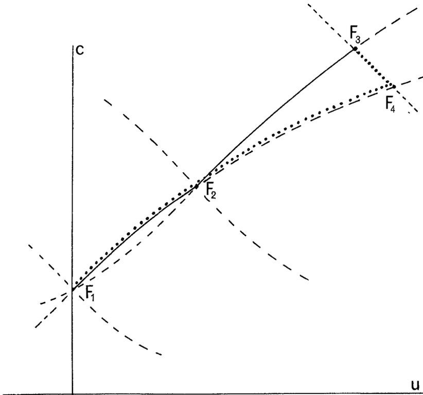
Figure 7. One bore catching another in the  $(u, c)$  plane. Bore  $B_1$  connects states  $F_1$  and  $F_2$ , bore  $B_2$  connects states  $F_2$  and  $F_3$ , the corresponding bore relations are shown by a continuous line. After the interaction the single bore  $B_3$  connects states  $F_1$  and  $F_4$  and a simple wave connects states  $F_4$  and  $F_3$  as indicated by the dotted line.
