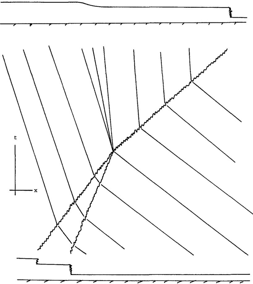
Figure 9 Diagram of  $(x,t)$  plane showing one bore catching another, with the C- characteristics and the bore paths shown. Below and above the diagram are representations of the initial and final states.
