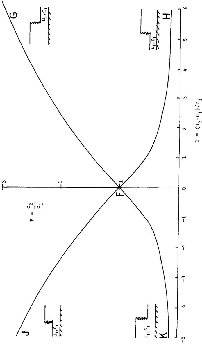
Figure 5. The bore relation, equation (17), in the  $(u, c)$  plane. The coordinates are given in terms of non-dimensional variables. The branch KFG represents a bore facing the  $+x$  direction, and the branch JFH represents a bore facing the  $-x$  direction, as indicated in the small sketches.
