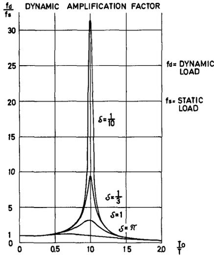
Fig. 2. Amplitude response curve for the damped oscillating system.
