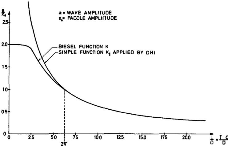
Fig. 4. Transferfunctions from paddle movement to wave profile.
