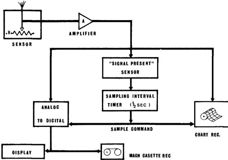
Fig. 3 Recording Technique
