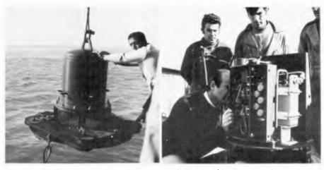
Fig.8 - CHATOU type pressure wave Fig.9 - Adjustment of pressure recorder (experimental stage in wave recorder (Huelva). January 1965 at the Tagus estuary).
