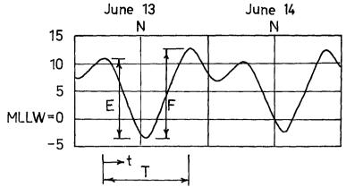
Fig. 3. Typical Tide Curves for Puget Sound, and Notation Definition
