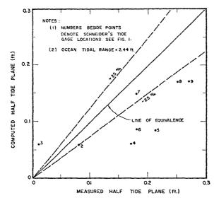
FIGURE 6 COMPARISON OF MEASURED AND COMPUTED HALF TIDE PLANES.
