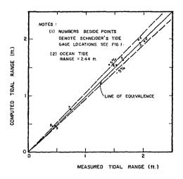
FIGURE 3 COMPARISON OF MEASURED AND COMPUTED TIDAL RANGES.
