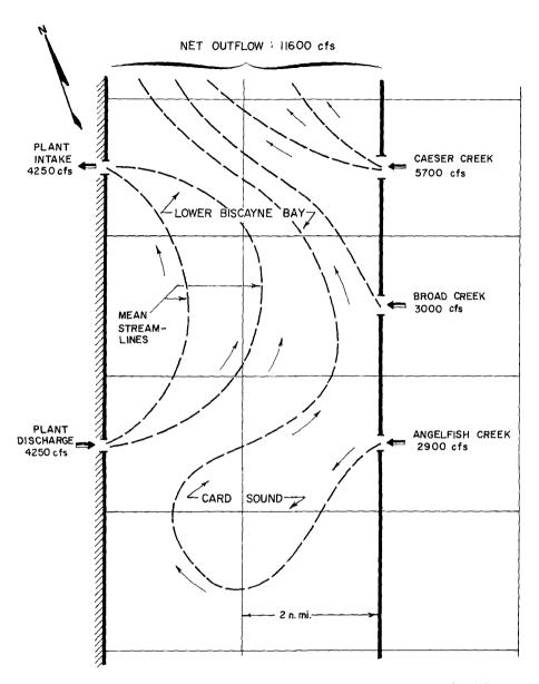
FIGURE IO MEAN STREAMLINES AND DISCHARGES ASSOCIATED WITH A PLANT FLOW OF 4250 cfs AND A SUSTAINED SSW WIND OF 15 KTS.
