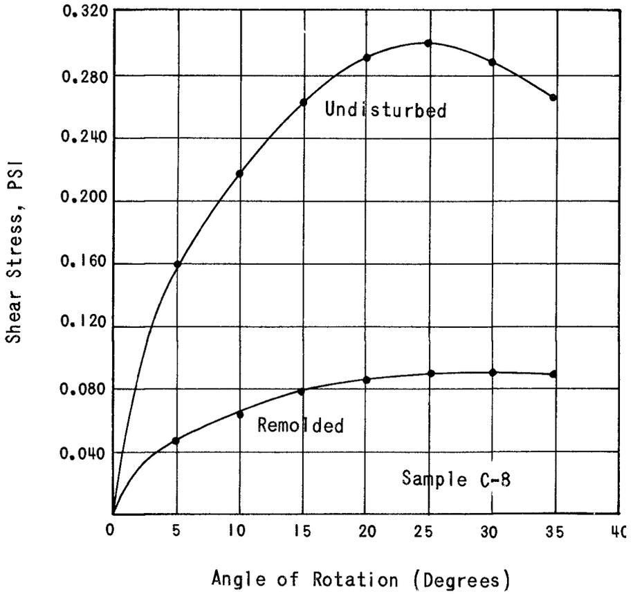
FIG. 6 RESULTS OF VANE SHEAR TEST
