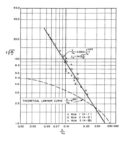
FIG. 2. PLOTTING OF EXPERIMENTAL DATA OF VELOCITY MEASUREMENT (SMOOTH BOTTOM)
