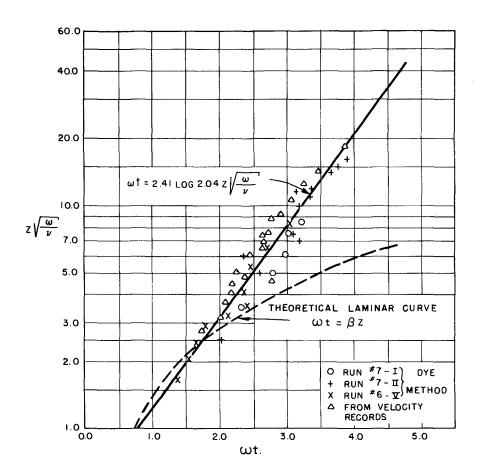
FIG. 3. PLOTTING OF EXPERIMENTAL DATA OF PHASE SHIFT MEASUREMENT (SMOOTH BOTTOM)
